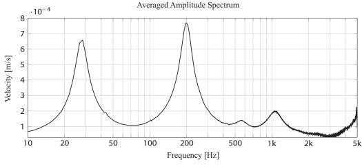
Operating deflection shapes corresponding to the local maxima of the spectrum at 28 Hz, 198 Hz, 530 Hz and 1077 Hz (from left to right).
