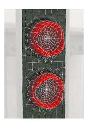
Operating deflection shapes of a **piezoelectric actor element (MFC)** fixed at one end. The diagram shows the average velocity of all scan points over the frequency. Below the first four modes are shown as the instantaneous amplitude of the displacement.
