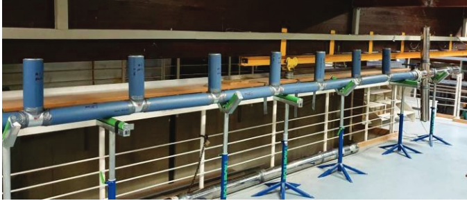
Figure 11: Test setup with seven quarter-wave resonator.
